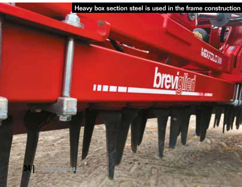
The five-metre machine has a 300hp central gearbox and runs 170hp side gearboxes
