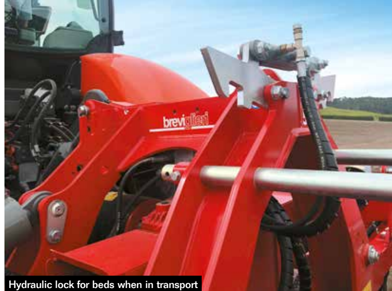
Hydraulic lock for beds when in transport
