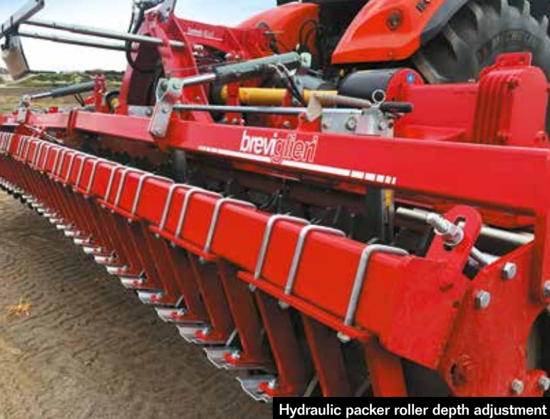
Hydraulic packer roller depth adjustment
