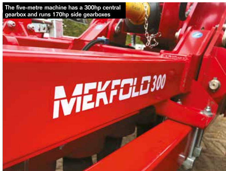
Heavy box section steel is used in the frame construction
