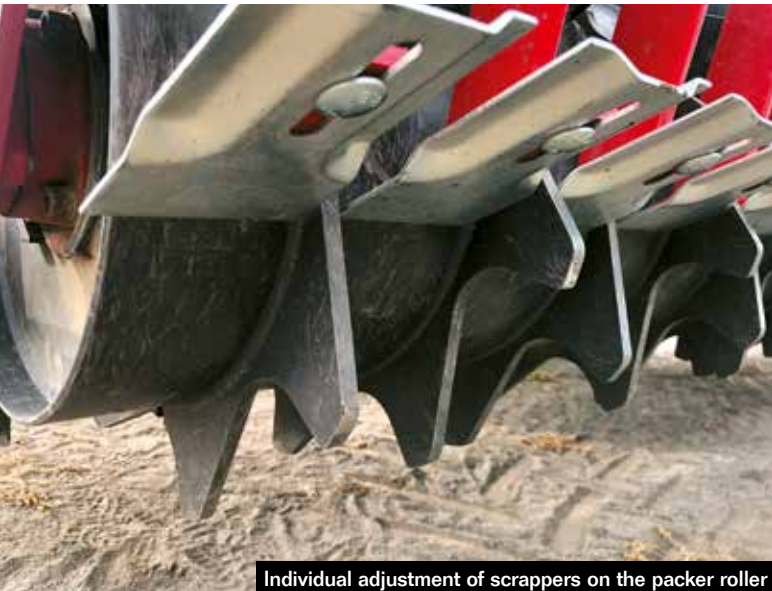
Individual adjustment of scrapers on the packer roller
