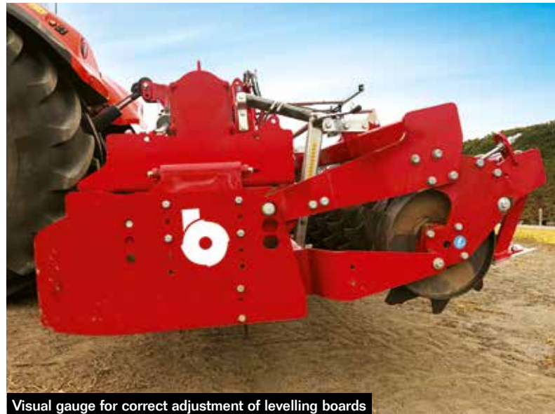
Visual gauge for correct adjustment of levelling boards
